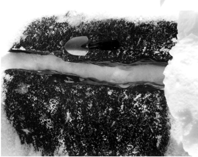
FIGURE 41. Tension crack on the drained lake flat with a 22 cm long trowel for scale.
